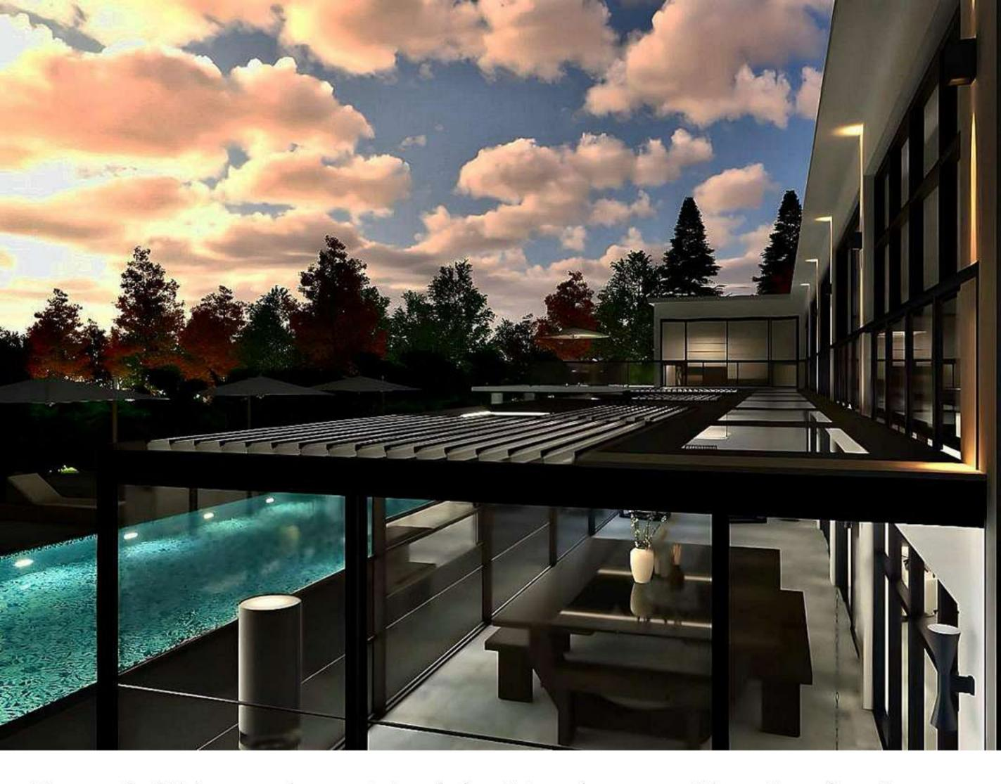
The roof of this pergola consists of aluminium louvres with various functions. Keep out the sun, let in a breeze or stay one step ahead of the rain? With the Somfy remote control, rotating the louvres in your pergola has never been so easy.
